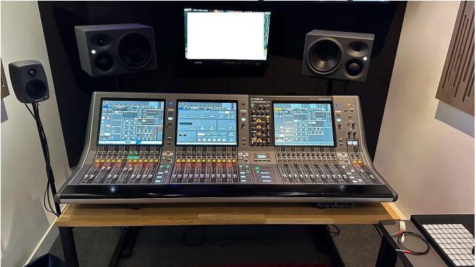
The CS-R5 control surface is the core component of RIVAGE PM5 system, with 96 kHz processing. The console has three touch screen and 12-faders bays for flexible setup and configuration. Touch panels are brought closer to the user, making them easier to reach. The weight is 92.6lbs (42kg) which is incredibly light.
